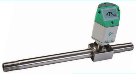
The CS flow sensor **VA 410** is based on the thermal mass flow principle. It measures volumetric standard flow over a wide measuring range. The result is pressure and temperature independent.
